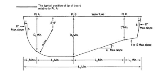
NOTE:  $L_4$  is a minimum dimension to allow sufficient length opposite the board. This may of course be lengthened to form the shallow portion of the pool.
