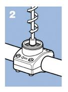
Cut hole in rigid PVC pipe using a power drill and the enclosed hole saw.
