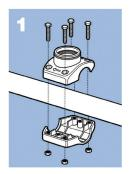
Turn pool pump off. Secure clamp assembly on the return line. For above-ground pools with corrugated pipe, use enclosed PVC adapter.
