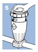
Thread the cartridge into the clamp, turn on pool pump and activate the cartridge. See manual for start up instructions.
