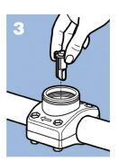
Insert the flow diverter into hole and snap it into place.
