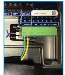
Figure 13. Pentair IntelliFlo/Hayward EcoStar Connection to Pump
