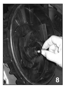
5. Install the rear bracket onto the drive unit using the bracket screw assemblies from the previous step. The handle of the rear bracket should be to the top of the drive unit. Tighten the screws securely.
