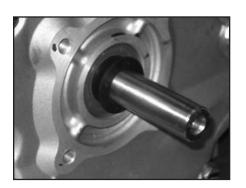
4. Screw the supplied 7/16-14 hex head cap screw into the impeller snout. As the bolt is tightened the impeller will be pried off of the shaft of the drive unit. Remove the 7/16-14 screw once the impeller has been removed from the drive unit.
