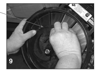
10. Install the volute (12702A) onto the rear bracket using the three volute screws (1-(12900), 20(12725)). Install the check valve (12705) onto the snout of the volute. The drive unit should be turned over a few times to check for clearance between the impeller and volute. A small amount of drag between the impeller and volute will cause no problem, however, if the drive unit will not turn over because of the lack of clearance a bracket shim may have to be used.
