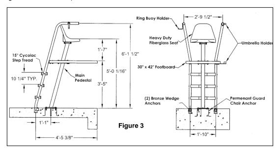
Read the entire manual before assembly to familiarize yourself with the product. Actual assembly of the chair, less the anchor installation, should take approximately 1 to 2 hours depending upon your experience. Two persons are helpful when assembling the main pedestal to the footboard and lifting into place on the anchor.
