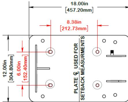
**Retrofit Hole Pattern Installations:** Use either of the two hole patterns shown below if replacing an existing swim lift on a pool deck. Utilize the hole pattern that matches your existing anchors.
