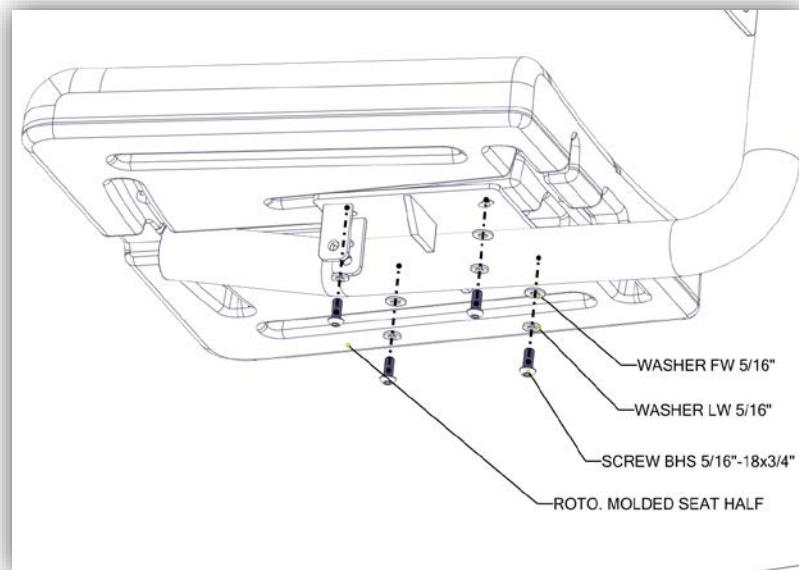
g. Attach the footrest to the bottom seat plate assembly using:
