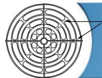
Internal ribs and walls are designed to optimize the impact-reducing capabilities of the disc, while keeping weight to the requisite level.
