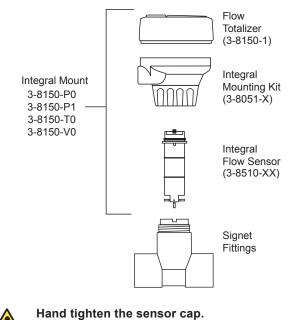
Hand tighten the sensor cap. DO NOT use any tools on the sensor cap or the cap threads and/or fi tting fl ange threads will be damaged,
