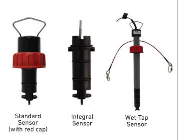
Simple to install with time-honored reliable performance, Signet 515 Rotor-X Paddlewheel Flow Sensors are highly repeatable, rugged sensors that offer exceptional value with little or no maintenance. The output signal of the Model 515 is a sinusoidal frequency capable of driving a self-powered flowmeter (Model 3-5090). The wide dynamic flow range of 0.3 to 6 m/s (1 to 20 ft/s) allows the sensor to measure liquid flow rates in full pipes and can be used in low pressure systems.
