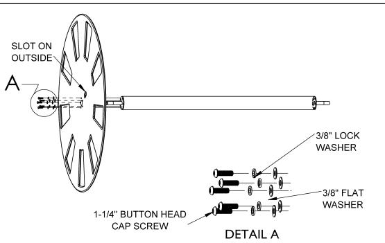
QUALITY: APPLY INCLUDED ANTI-SEIZE TO STAINLESS-STEEL THREADS WHEN FASTENING. THIS PREVENTS THE SCREW FROM GALLING.
