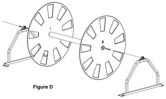
4) Slide PVC tube around the side support rail.
