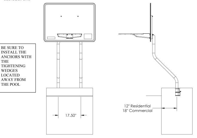
NOTE: Each anchor socket has a removable cap, which needs to be removed before inserting the assembly. The cap can be removed by inserting a small flat blade screwdriver into the center hole of the anchor cap and pulling up. When removing the basketball assembly from the anchors make sure to place the caps in the anchors.
