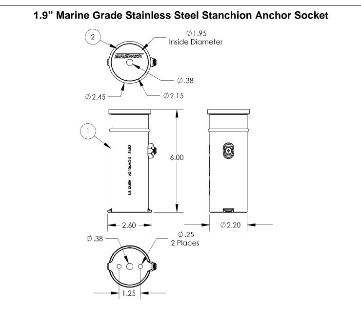
**Specification:** The 1.9" Marine Grade Stainless Steel Stanchion Anchor Socket (Item 1) is made of 316 stainless steel and is 6" (152.4mm) deep, allowing for mounting 1.90" O.D. (48.3mm) fixtures without the use of a wedge assembly. The anchor is tapped for the provided #10 UNC brass grounding screw. A marine grade stainless steel cap (Item 2) is provided to mount flush with the deck when the fixture is removed.
