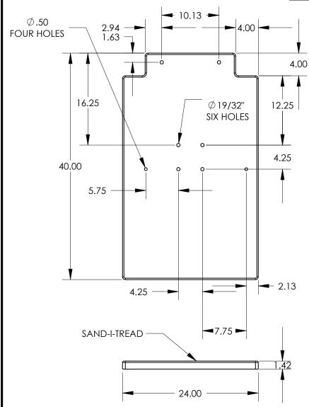
**UNLESS OTHERWISE SPECIFIED** DIMENSIONS ARE IN INCHES, **TOLERANCES ARE:** FRACTIONAL: ..... ± 1/16 ANGULAR: ..... ±1°
