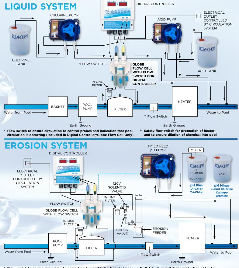
\* Flow switch to ensure circulation to control probes and indication that pool circulation is occurring (Included in Digital Controller/Globe Flow Cell Only) \*\* Safety flow switch for protection of heater and to ensure dilution of chemical into pool
