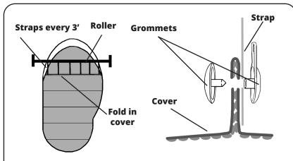
For odd shaped pools, pinch the cover and attach the strap as shown. Attach the cut cover to the roller with the blue straps (see grommet detail) by folding the cover in a straight line as shown in the diagrams. Ensure that the fold in the cover is straight.
