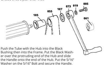
**NOTE** do not over tighten this bolt as it will make it hard to rotate the Handle. Repeat this on the other end of the unit and use the Knob in place of the Handle.
