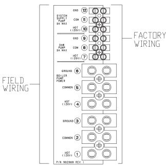
Fig. 20: Wiring Electrical Connections
