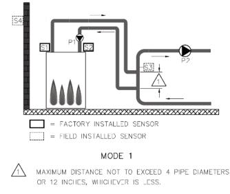
Fig. 13: MODE 1 - Single Boiler with Primary/Secondary Piping
