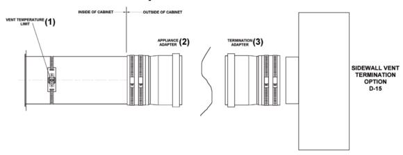
Fig. 31: Centrotherm Polypropylene Vent Adapter
