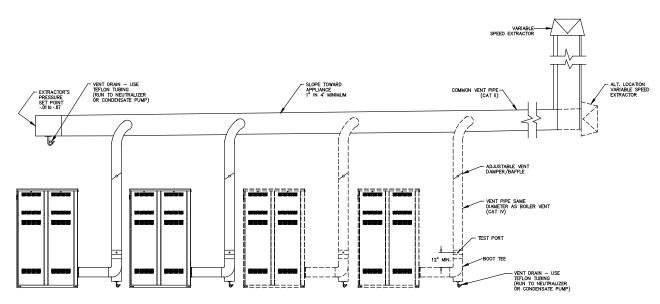
Note: Units rotated 90° for clarity. Typical multi-unit installations have the heaters installed side-by-side. Extractor is required.
