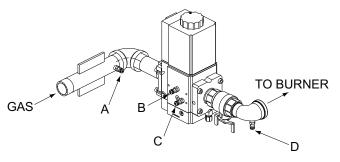
Fig. 46: Gas Pressure Measurement Locations
