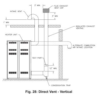
**CAUTION:** This venting system requires the installation of a condensate drain in the vent piping per the vent manufacturer's instructions. Failure to install a condensate drain in the venting system may cause a non-warrantable failure. Condensate is acidic and highly corrosive.
