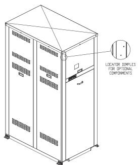
Fig. 24: Locator Dimples for Optional Components
