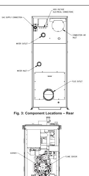
FRONT OF HEATER Top panel, blower and gas train omitted for clarity Fig. 4: Component Locations – Top
