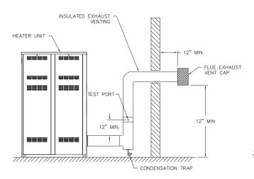
Fig. 25: Horizontal Through-the-Wall Venting
