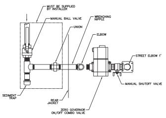
Fig. 19: Gas Supply Connection
