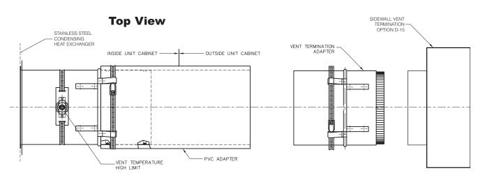
Fig. 30: PVC Vent Adapter
