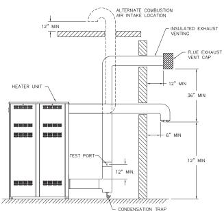
Fig. 27: Horizontal Through-the-Wall Direct Venting
