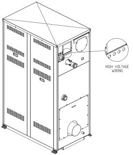
Fig. 23: Wiring Location
