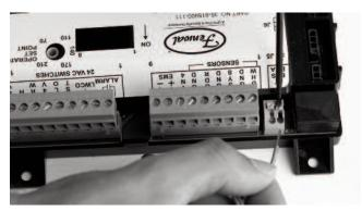
Fig. 26: FT\_BUS Wire Connection
