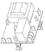
Fig. 41: Low Water Cut-Off
