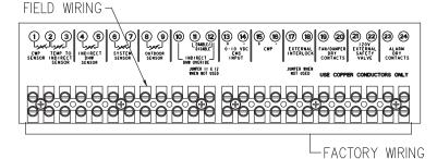
Fig. 25: Low Voltage Field Wiring
