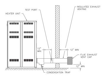
Fig. 26: Alt. Horizontal Through-the-Wall Venting
