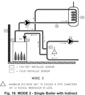
ig. 16: MODE 3 - Single Boiler with Indirect on Boiler Loop
