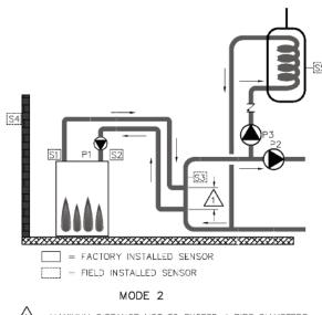
MAXIMUM DISTANCE NOT TO EXCEED 4 PIPE DIAMETERS OR 12 INCHES, WHICHEVER IS LESS.
