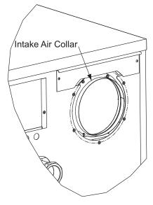
Fig. 12: Install the Intake Air Collar
