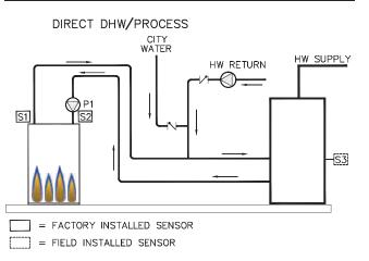
Fig. 17: WH Units - Single Water Heater with Tank H Units - Single Boiler with Process Tank
