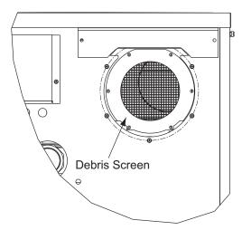
Fig. 11: Remove the Debris Screen
