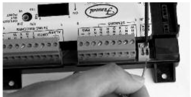
Fig. 23: FT_BUS Wire Connection
