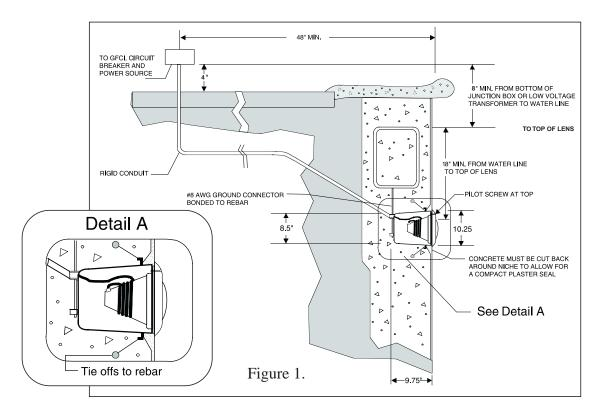
The niche is properly electrically bonded and grounded using the No. 8 AWG ground connector located at the rear of the niche, see Figure 1.
