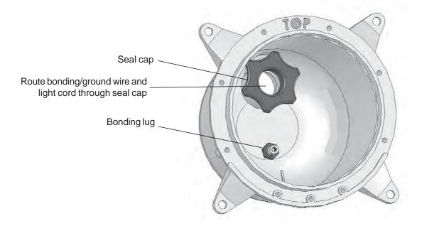
6. Grasp the seal and spread the smaller opening, and clip onto the for bonding/ground wire. Spread the larger opening, and clip onto the light cord as shown. Orient the seal pins facing outward.
