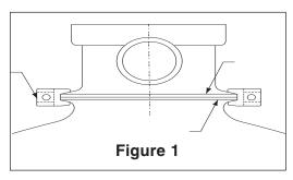
The plastic clamp can now be installed. Place the clamp half over the valve flange and the tank flange as shown in Figure 1. Insert the clamp screws and nuts into the clamp making sure that the nuts are located in the special hexagonal retainer slots on the clamps. See Figure 2.
