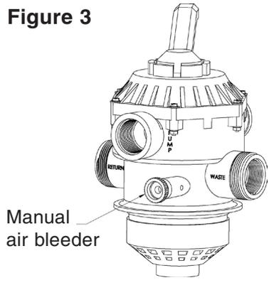
8. Turn the pump off and set valve to “Filter” position. Be sure that all pool suction and return lines are open so that water is free to flow from and to the pool.
