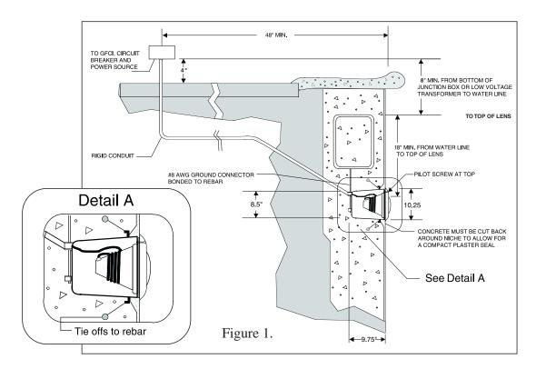
The niche is properly electrically bonded and grounded using the NO. 8 AWG ground connector located at the rear of the niche, see Figure 1.
