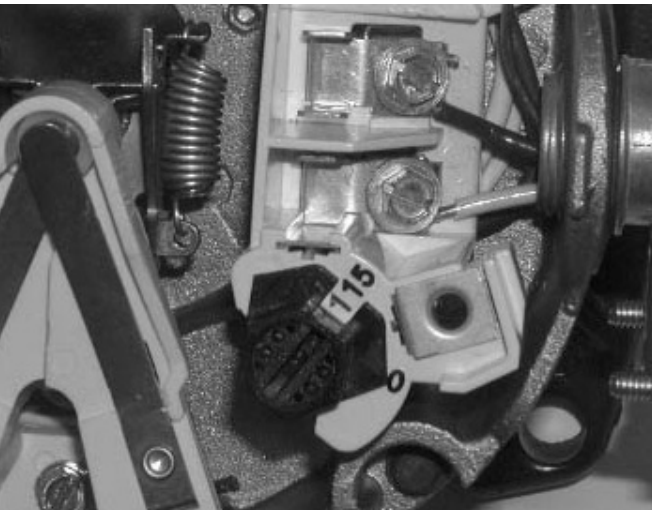
Figure 4: Motor Set for 115 Volt Operation
