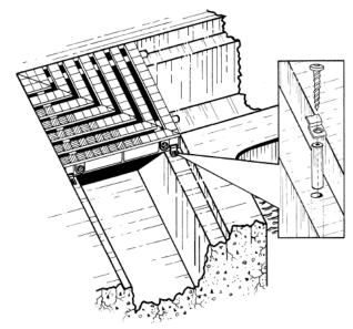
Note- any corner that is not a true 90 or 45 degree corner Will require a Template Kit. Kits are issued by the Manufacturer And returned by the Customer for factory fabrication
