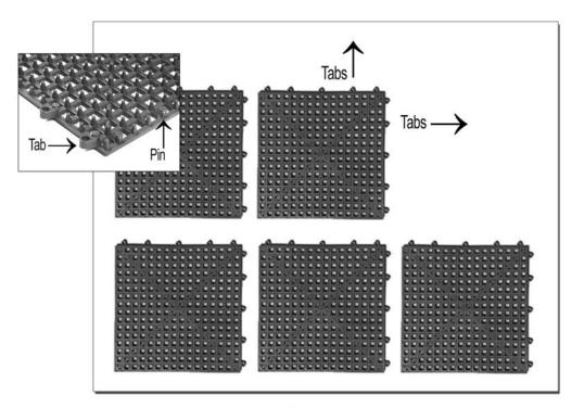
Size up the area you wish to cover. Layout the Dri-Dek Tiles™in the desired configuration. Point the outer tabs of the Tiles in the same direction. Dri-Dek Sheets™and Rolls™will interlock in an identical manner. For large areas, install in independent sections approximately 10' x 10' to allow for ease of cleaning, maintenance and normal expansion and contraction from temperature variations.
