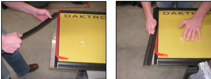
Figure 21: Applying Vinyl Edge Cover
