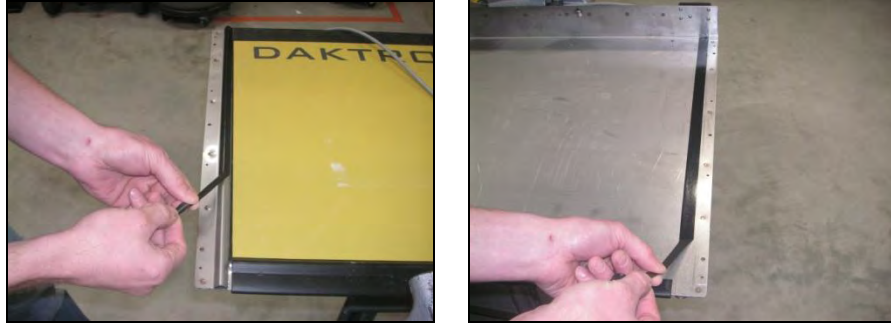
Figure 12: Removing Old Tape
