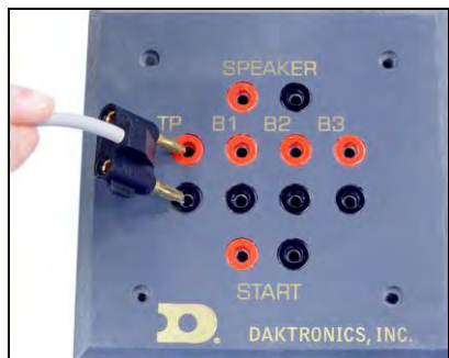
Figure 9: Individual Lane Deck Plate
