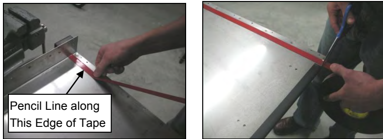
Figure 15: Applying & Cutting New Tape (Rear)
