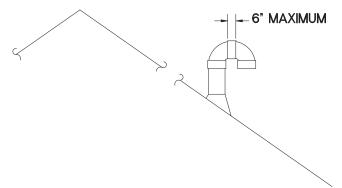
Figure 26 – Vertical Rooftop Air Inlet
