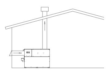
Figure 14 - Sidewall Combustion Air Inlet
