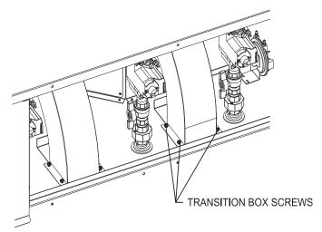
Figure 53 – Loosening Fan Transition Box Screws
