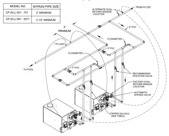
Figure 37 - Heaters are Beyond 15 feet of Pool Piping
