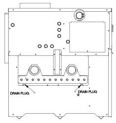
Figure 3 - Draining Pool Heater
