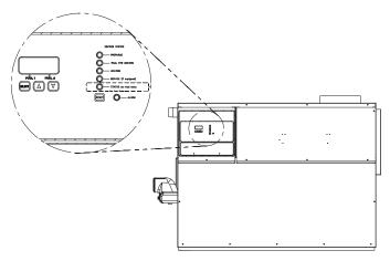
Figure 49 – Exterior Control Panel with Operation/Diagnostic Lights and LCD Display
