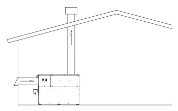
Figure 18 – Vertical DirectAire Installation with Sidewall Combustion Air Inlet
