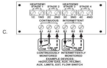
Figure 40 (A-C) - Terminal Strip Connection
