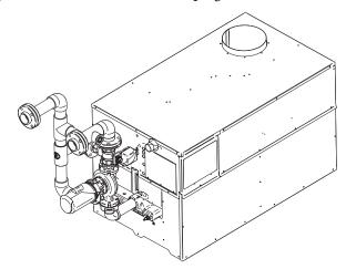
Figure 45 – Horizontal Pool Heater Piping
