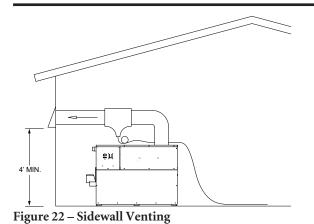
⚠ WARNING: Do not combine the flue from this unit with the vent from any other appliance. Do not combine flues from multiple appliances into a common vent. The flue from this unit must be a dedicated stack.
