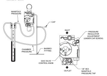
Figure 31 - Measuring Net Manifold Gas Pressure
