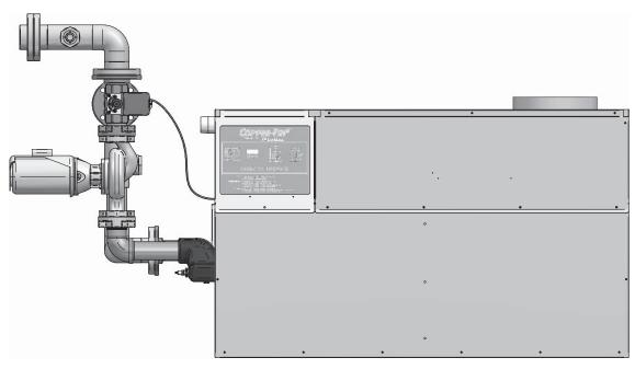
Figure 1A – Standard Horizontal Piping Loop
