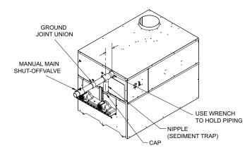
Figure 28 - Gas Line Connection
