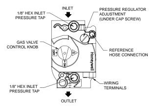
Figure 43 – Combination Gas Valve
