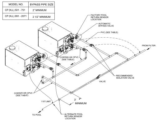
Figure 36 - Heaters are within 15 feet Perpendicular of Pool Piping
