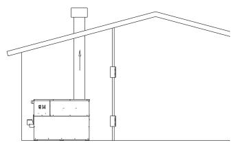
Figure 8 - Outside Combustion Air Through Ducts
