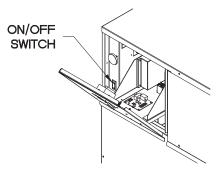
Figure 42 - ON/OFF Switch
