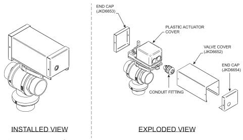
Figure 32 – 3-Way Valve Cover
