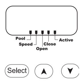
Figure 46 – Temperature Control Display and Programming Keys
