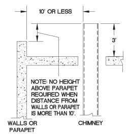
Figure 13 – Vent Termination from Flat Roof More Than 10' from Parapet Wall
