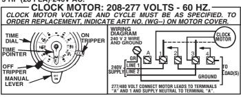
**WIRING INSTRUCTIONS:** To wire switch follow diagram above. Use solid or stranded COPPER **only** wire with insulation to suit installation. See gauge selection table for normal service applications. To make power connections remove 1/2 inch of insulation from wire ends. Insert bare ends of wire under the pressure plate of terminals. Use 3/16 or larger screwdriver to tighten terminal screws firmly. (25 lb-in minimum).
