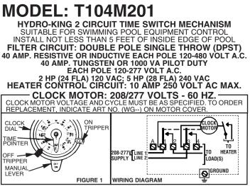
To wire switch follow diagram above. WIRING INSTRUCTIONS: Use solid or stranded COPPER wire with insulation to suit installation. See gauge selection table for normal service applications. To make power connections see illustration below. Use 3/16 or larger screwdriver to tighten terminal screws firmly. REPLACE INSULATOR BEFORE TURNING ON ELECTRICITY. NOTE: MOTOR VOLTAGE AND CYCLE (HZ.) MUST BE AS SPECIFIED ABOVE.
