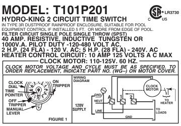
WIRING INSTRUCTIONS: To wire switch follow diagram above. Use solid or strand COPPER only wire with insulation to suit installation. See gauge selection table for normal service applications. To make power connections remove 1/2 inch of insulation from wire ends. Insert bare ends of wire under the pressure plate of terminals. Use 3/16 or larger screwdriver to tighten terminal screws firmly. (25 lb-in minimum). BEPLACE INSULATOR BEFORE TURNING ON FLECTBICITY.
