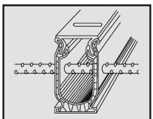
This drain is not designed to be used as a full expansion. Stegmeier LLC requires that a 3/8" coated or non-metallic rebar be placed every 36 inches, midway in the drain to prevent damage due to concrete deck movement.
