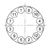
I NOTE: Bolt length based on connecting two (2) LASCO flanges, two (2) flat washers, and nut. Actual Bolt lengths required and torque values necessary to seal will vary based on type of equipment being joined. Adjustments will need to be made to when assembling flanges to accommodate valves and other equipment.
