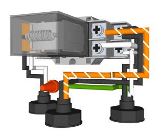
$\begin{array}{l} A = \text{Female Piptail, Plug Saline C 6.0} \\ B = 120\text{v to the Controller} \\ C = \text{Power Cable, } 120\text{v} \end{array}$
