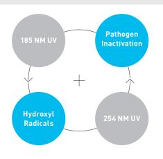
Dual-wavelength amalgam lamps produce germicidal UV.
