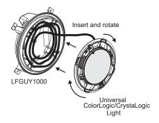
Install either the white or gray plastic trim ring by gently snapping all four trim ring tabs to the four cutout locations on the light flange. Note that the gray trim ring with the mounting screw hole should be used if the stainless steel trim ring will be installed over it (see next section below).
