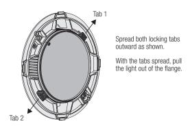
This method can also be used if the light requires replacement after installation. There is no need to remove the flange from the niche; just remove the light using the method above.
