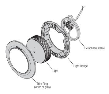
Note that the light and flange are shipped from the factory as an assembly. For most installations, it will be easier to keep these parts together. If your installation requires you to remove the light from the flange, refer to the diagram below.
