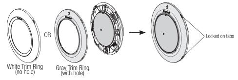
**Stainless Steel Trim Ring Installation (optional)** - position over the light and gray plastic trim ring and insert the two hooks on the bottom with the two recesses on the plastic trim ring. Tilt the stainless steel trim ring toward the light and then finish the installation by hand-tightening the screw into the hole at the top of the stainless steel trim ring. Be careful not to over tighten.
