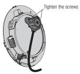
After fully seating the connector, use a screwdriver to secure. Just snug the fasteners and be careful not to overtighten (screw torque does not affect water tightness). To remove the cable, fully loosen the screws, push down on the clip to release and then pull the connector out of the socket.
