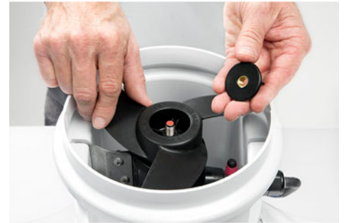
3. Once the prop nut is off, you will be able to remove the propeller from the motor shaft by lifting it up.
