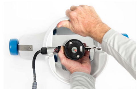
3. Working from the top, gently pry the head halves apart and lift the motor assembly up and out of the vacuum head. (Reverse this procedure to install the motor/cord assembly).
