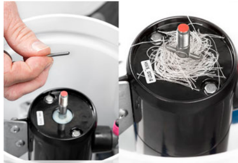
5. With the pin out, clean any debris that may be wrapped around the motor shaft.
