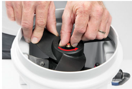
2. To remove the prop nut: Hold the propeller with one hand and turn the prop nut counter-clockwise with the other hand.
