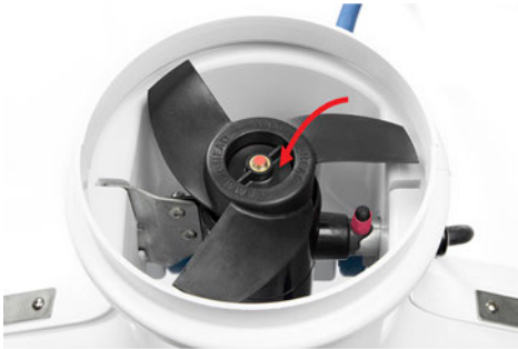
1. Locate the prop nut in the center of the propeller. It looks like this:
