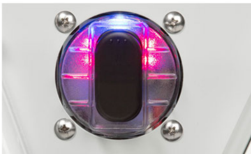
3. In WIRING FAULT MODE the switch will flash red and blue (older models may flash red only). This indicates that there is a wiring and/or connectivity problem. Check ALL connections.
