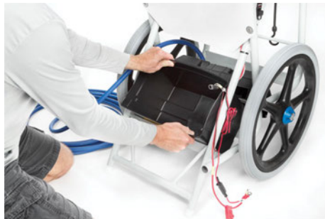
2. Tilt the battery box forward and pull the wires out to the side. (Additional parts may be stored inside the battery box for shipping).
