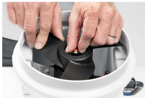
2. Remove the propeller nut, propeller, and propeller pin. (Refer to REMOVING THE PROP guide for instructions).
