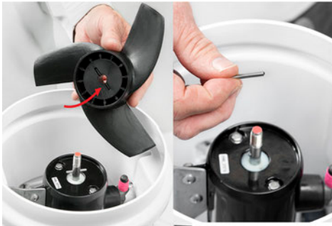
4. Locate the groove on the bottom of the propeller and the prop pin that goes through the shaft. (When re-installing the propeller, the prop groove must be seated on the pin). Remove the pin from the shaft. DO NOT LOSE THE PIN!
