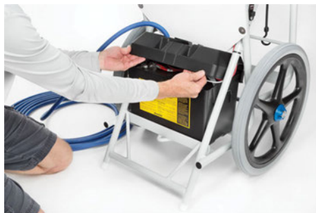
5. Tilt the battery box back into place using the handle on the battery. Pull the battery box lid back through the cart to the front and replace the cover.
