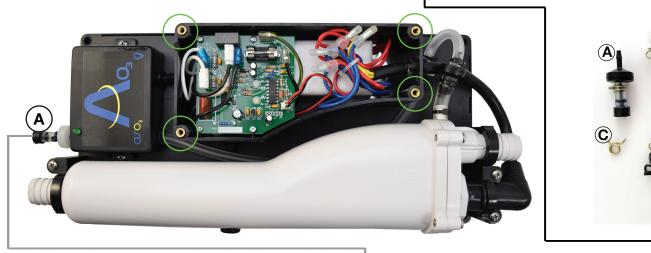
Step 2: Remove and replace the air inlet with check valve B. Attach new clamp securely C .
