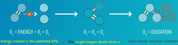
Energy created in the patented APG cell splits molecular oxygen  $(O_2)$  into atomic oxygen  $(O_1)$ .
