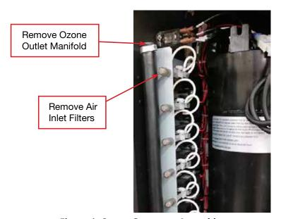
**Figure 1. Ozone Generator Assembly**
