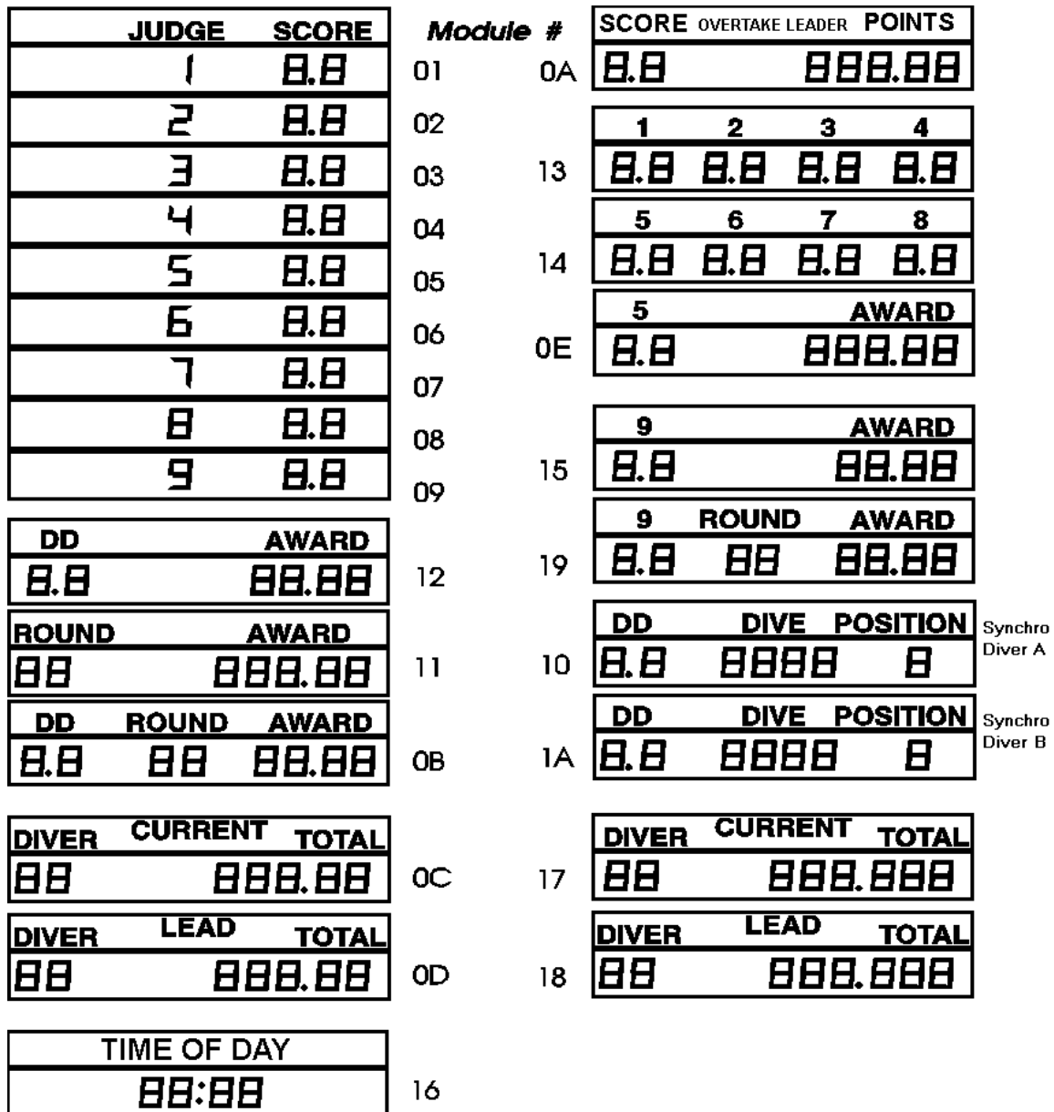
Figure 3-G shows the diving scoreboard modules with signage installed and module numbers indicated.
