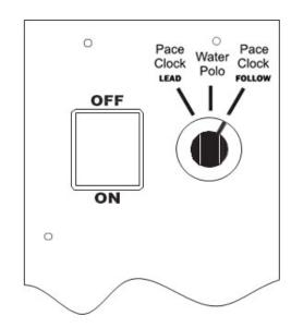
After the dial has been in the same channel setting for 4 seconds, the clock will display the firmware revision, and then the current mode. At this point, the dial changes the mode. The dial will change only the mode until the clock is turned off and then on again.
