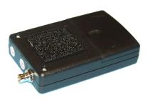
Figures 3 & 4: hook and loop fastener on Infinity and on Dolphin Starter
