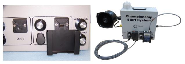
Attach the cable and adapter between the Dolphin Starter and the Timer Start jack on the ChampStart. **NOTE**: you must **unlock** the locking mini BNC connector when disconnecting from the Dolphin Starter or you will damage your cable.
