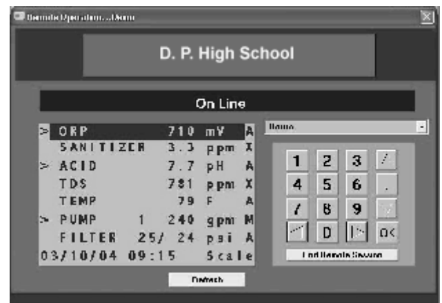
Figure 41 - CHEMCOM™ Remote Operation Screen
