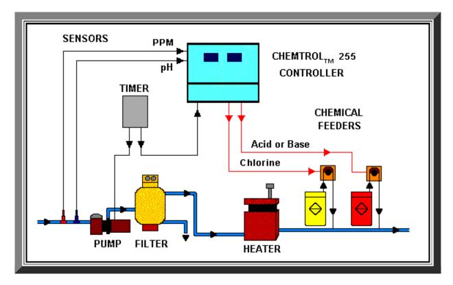
Installation of the CHEMTROL<sup>®</sup> 255 is as easy as 1-2-3.
