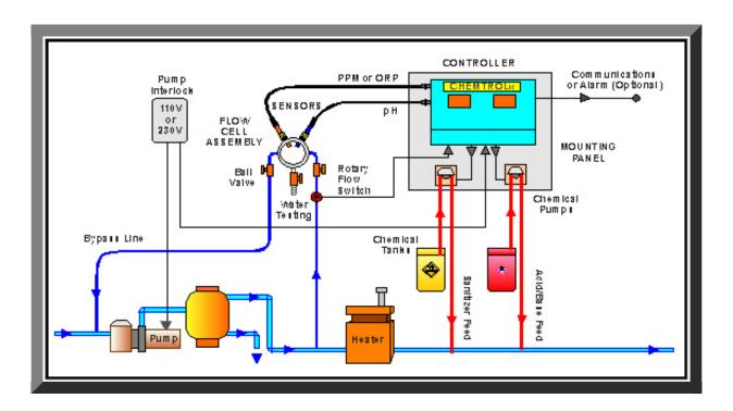
The FCA includes a see-through cell with a plastic cover that regulates the flow of water and allows the operator to see the tip of the sensors.
