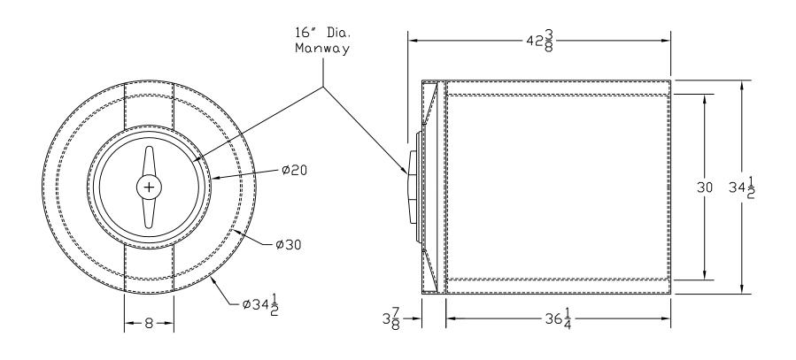
ALL DIMENSIONS SHOWN ARE OUTSIDE PART DIMENSIONS IN INCHES,AND VARY BY THE STANDARD ROTATIONAL MOLDING TOLERANCE OF 2% TO 3%.
