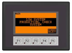
Example with Fault Message (Flashing Amber Backlight)
