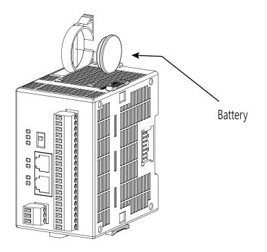
Figure 8: Battery Replacement
