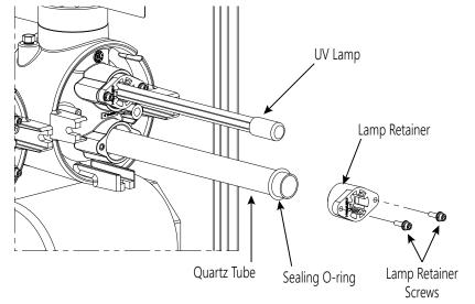
Figure 6: UV Lamp and Quartz Tube Removal
