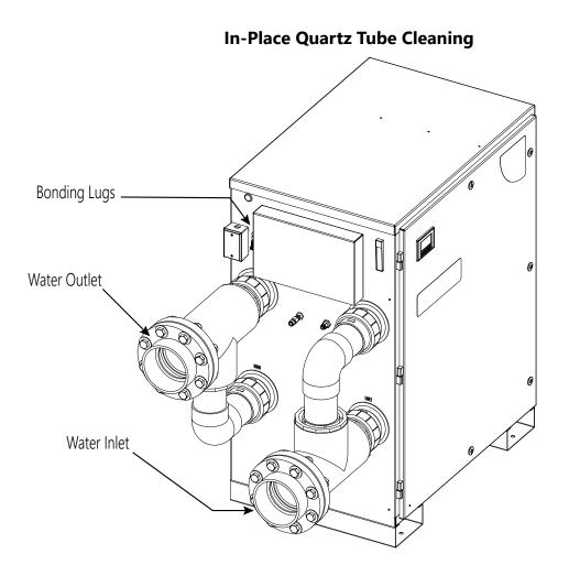
The AOP Pro quartz tubes may be cleaned without removing them from the vessel.
