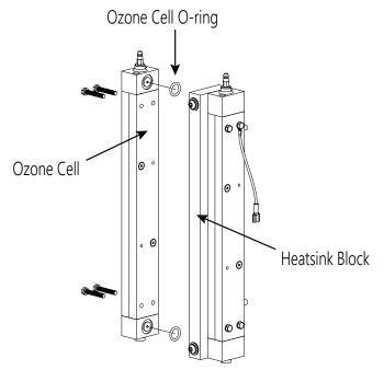
Figure 5: Ozone Cell and O-ring Service
