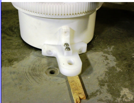
USE A SHIM UNDER THE TAB
