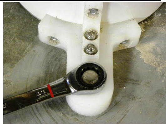
THEN TIGHTEN WITH 3/4" WRENCH TIGHTEN UNTIL BOLT IS FLUSH DO NOT OVERTIGHTEN!
