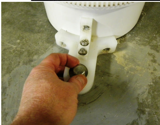
INSTALL BOLT & THREAD BY HAND
