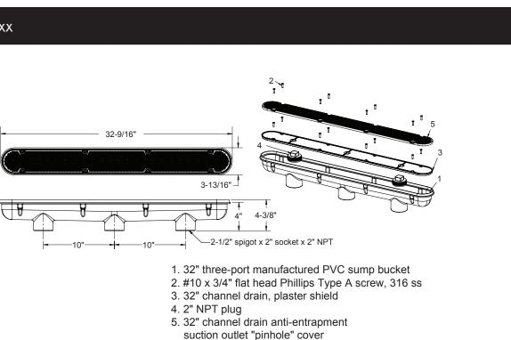
Note: unless otherwise specified, plaster shield and screws to be removed after installation.
