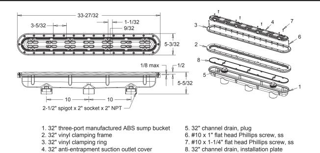
Note: unless otherwise specified, plaster shield and screws to be removed after installation.
