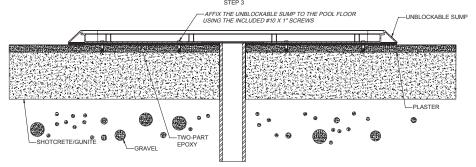
The sump must be permanently and securely affixed to the pool floor using epoxy around the entire edge and the enclosed plastic anchors or optional brass anchors. Once this is completed, the sump becomes a permanent part of the pool structure, creating an unblockable drain. The drain cover is then affixed to the sump using the designated screws.
