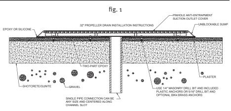
The sump must be permanently and securely affixed to the pool floor using epoxy around the entire edge and the enclosed plastic anchors or optional brass anchors. Once this is completed, the sump becomes a permanent part of the pool structure, creating an unblockable drain. The drain cover is then affixed to the sump using the designated screws.
