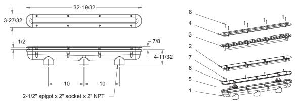
1. 32" three-port manufactured PVC sump bucket 2. 32" leaf trap insert 3. 32" leaf trap cover 4. 32" channel drain "buzz top" cover 5. 2" NPT plug, qty 2 6. 32" channel drain, plaster shield
