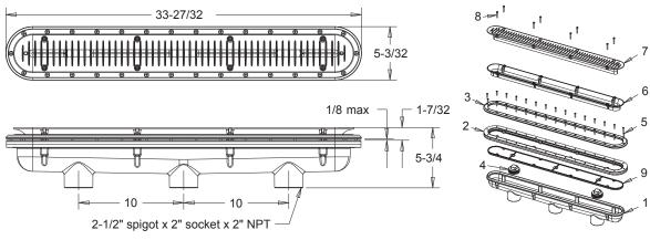
1. 32" three-port manufactured ABS sump bucket 2. 32" vinyl clamping frame 3. 32" vinyl clamping ring 4. 32" channel drain, plug 5. #10 x 1" flat head Phillips screw, ss
