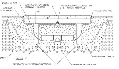
\* AT IAPMO (A NATIONALLY RECOGNIZED TESTING LAB), ALL AQUASTAR SUCTION OUTLET COVERS HAVE BEEN TESTED WITH 3" DEEP SUMPS (UNLESS OTHERWISE INDICATED).
