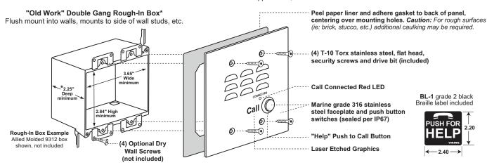
\* Caution: Excessive wire length and/or using a rough-in box with inadequate depth can apply force to the circuit board causing physical damage.
