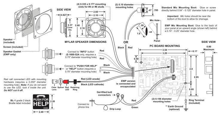
\* Important: If installing the EWP version outdoors, apply a non-corrosive silicone to back side of LED and push button switches after making all connections and testing. Completely encapsulate exposed switch connections (terminals/stripped wires) and bare wire connections.
